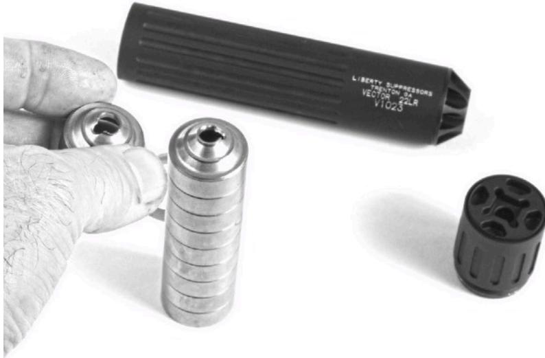
port opposing the first one. There is a little step in the baffle so the next one will center easily on it. Once ten baffles are stacked, add the blast chamber spacer ring to the top.
