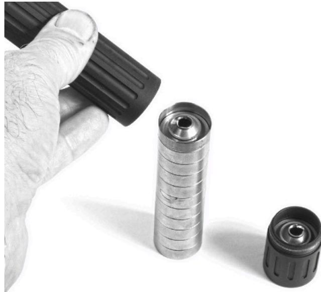
6. Should you choose to install the extension tube, screw it in hand tight until it seats against the baffle stack in the tube and takes up all the slack. Next drop in the last two baffles with the nose facing the same direction as the other ten, in the main tube, and alternate the notched ports similarly.
