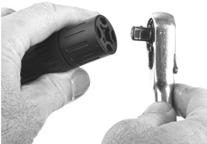
5. Use the ratchet to remove the front cap (there is a square recess that is there for the ratchet) from either the extension housing or the end of the silencer(short configuration).
